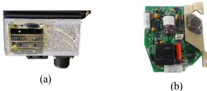
Fig. 2. The inside structure of the voltage controller (a) Molding structure (b) The circuit board
