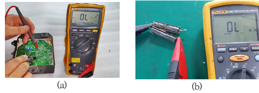
Fig. 3. The results of the functional failure tests (a) The measurement of the zener diode (b) The measurement of the resistor
