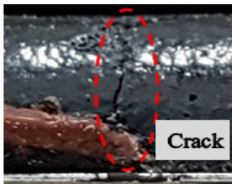
Fig. 7. The crack of the resistor occurred in temperature saturation test
