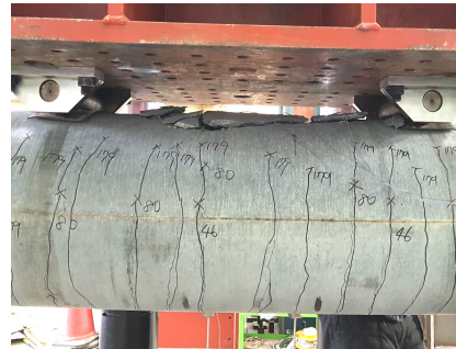
Fig. 9. Concrete cracks in sample RC500-F-NJ after the bending test
