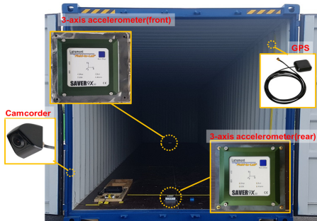
Fig. 2. Installation of the measurement sensors
