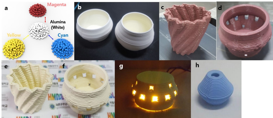
Fig. 5. Various ceramic 3D printing structures with ceramic pigment. (a) Schematic of high temperature ceramic pigment (b) 3D printed alumina structure (c) and (d) 3D printed structure with magenta pigment (e) and (f) 3D printed structure with yellow pigment (g) application of 3D printed Lamp structure with LEDs (h) 3D printed structure with cyan pigment
