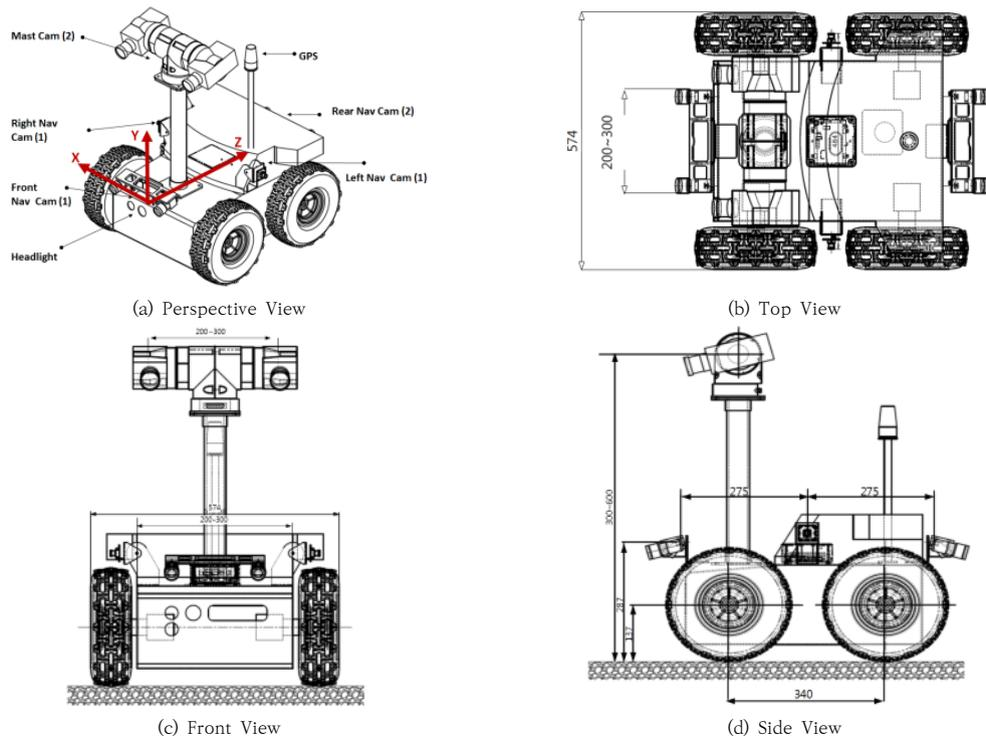
Fig. 1. Concept Design of Rover's Camera System
