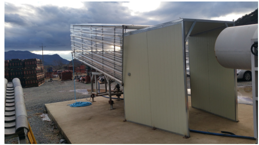
Fig. 17. Water infiltration test apparatus
