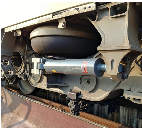
Fig. 9. Replacement of yaw damper
