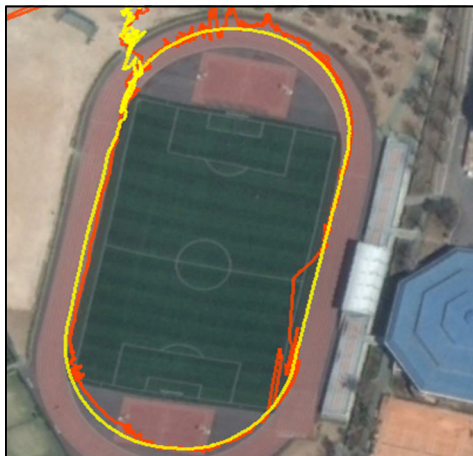
Fig. 7. Comparison of drone tracking results obtained with single GPS (red line) and with DGPS (yellow line)
