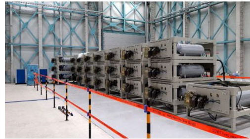
Fig. 3. Freight train brake test bench
