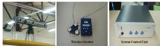
Fig. 3. Motion Capture System
