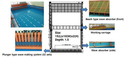
Fig. 1. Schematic and Photo of 3D Wave Model Basin
