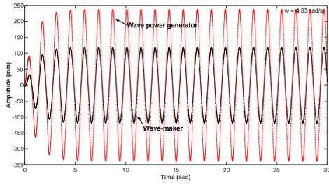
Fig. 6. Amplitude of the Cylinder-type Buoy and the Incident wave versus time at 4.83 rad/sec frequency
