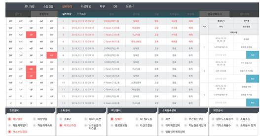
Fig. 7. Facility status screen of integrated fire protection system
