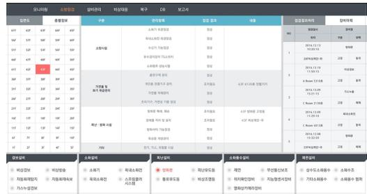
Fig. 6. Diagnosis results screen of integrated fire protection system
