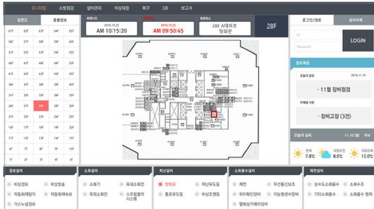
Fig. 4. Main screen of intelligent integrated fire protection system
