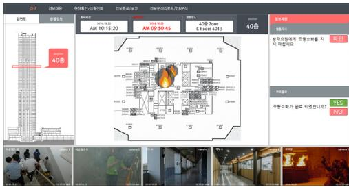
Fig. 9. Main screen of the emergency response system
