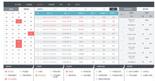
Fig. 8. History inquiry screen of integrated fire protection system
