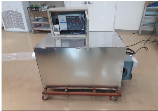
Fig. 2. Carbon dioxide supply system
