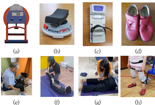
Fig. 1. Measurement devices and methods. (a) grip force dynamometer (b) muscle manual testing dynamometer (c) toe grip force dynamometer (d) inertia-sensor built-in shoes (e) toe grip force testing (f) gluteus medius testing (g) gluteus maximus testing (h) gait testing
