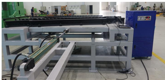
Fig. 16. Hydraulic actuator in operation
