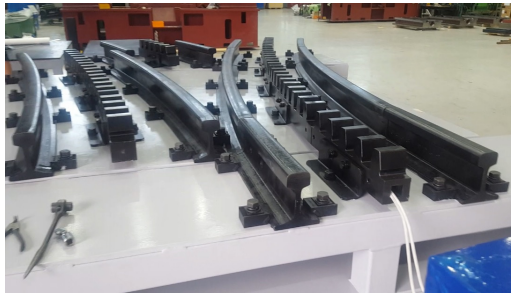
Fig. 15. Prototype switching device with induction heating pipe in test
