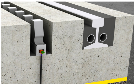
Fig. 13. Induction heating pipe in embedded concrete rack track
