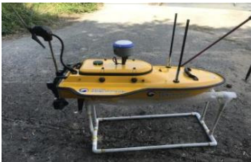
Fig. 2. Unmanned Survey Vehicle(USV)
