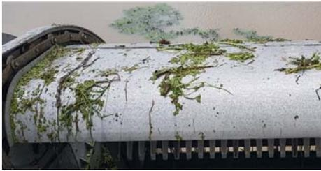
Fig. 3. Attached narrow trash on the trash screen
