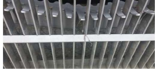
Fig. 2. Failure rake caused by jamming
