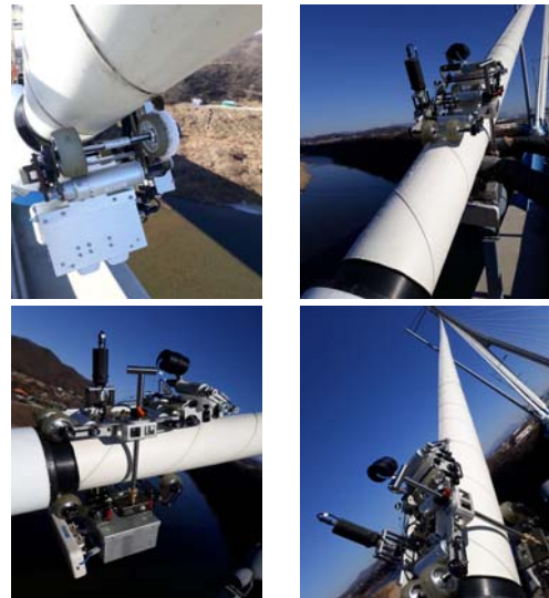
Fig. 5. Testing snow removing robot on the cable
