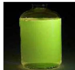
Fig. 2. Fluorescent dye for detection of engine oil leakage
