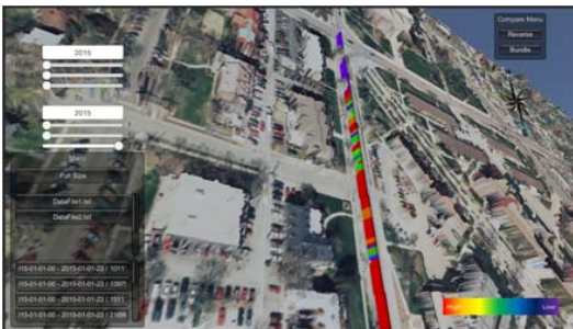
Fig. 9. Annual solar irradiation visualization for each panel in candidate site number 2
