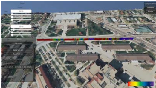
Fig. 8. Annual solar irradiation visualization for each panel in candidate site number 1
