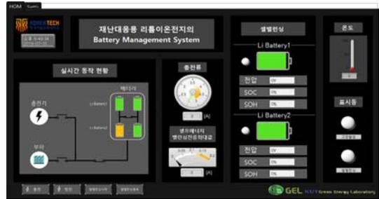
Fig. 7. Main menu of BMS based on Labview S/W
