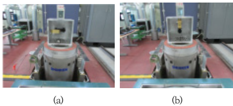
Fig. 10. Vibration endurance tests (a) Transverse (b) Longitudinal
