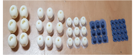
Fig. 2. Coarse aggregates made with 3D printer
