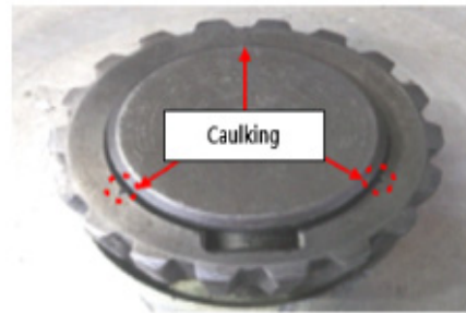
Fig. 14. Shape of caulking work for hub
