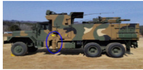
Fig. 1. Mounting position of Launch Support Device (LSD)
