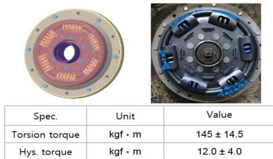
Fig. 15. The configuration and specifications of damper coupler
