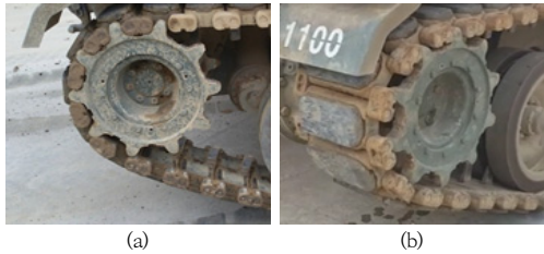
Fig. 4. Influence of tension between sprocket and track
