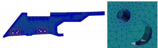
Fig. 9. BRU Pin Hole : Critical Area of Pylon
