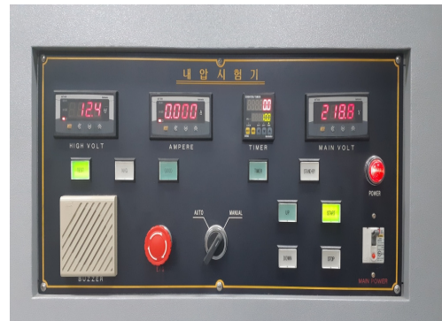
Fig. 14. AC Breakdown Voltage Equipment
