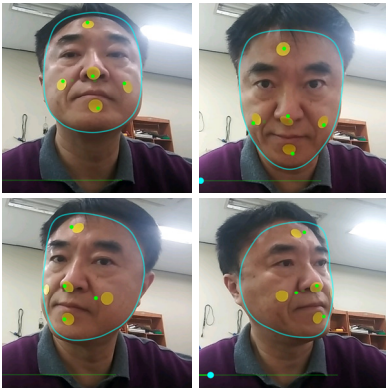
Fig. 7. Display of ultrasonic-irradiation locations according to face poses (ultrasonic irradiation on a 19mm pad)
