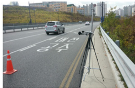
Fig. 3. Measuring noise level at the roadside
