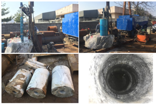
Fig. 13. Uneven excavation for production of specimens
