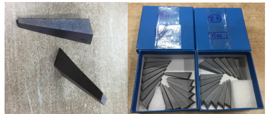
Fig. 9. Prototype for drilling bite tips
