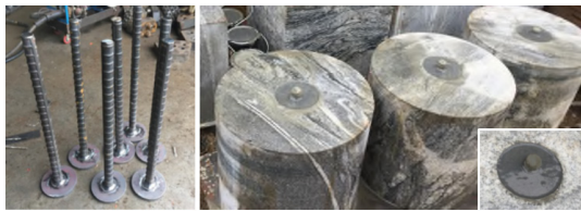
Fig. 14. Rock bolt and grouting of specimens
