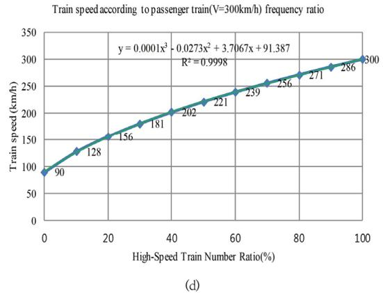
Fig. 2. Train operation speed comply with high speed train operation ratio
