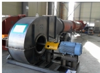
Fig. 13. Photograph of model blower installation.
