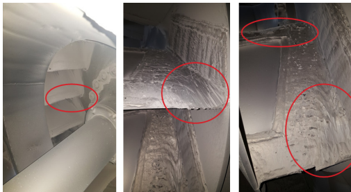
Fig. 10. Photograph of erosion field test result (non deflector type blower).
