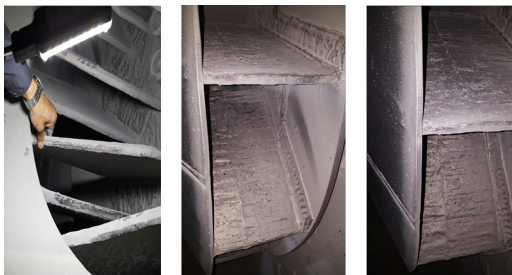
Fig. 11. Photograph of erosion field test result (dust deflector type blower).
