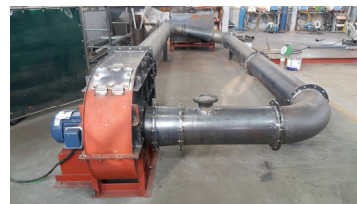
Fig. 6. Photograph of blower erosion tester.
