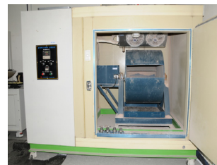
Fig. 2. LA Abrasion Tester in Constant Temperature Chamber
