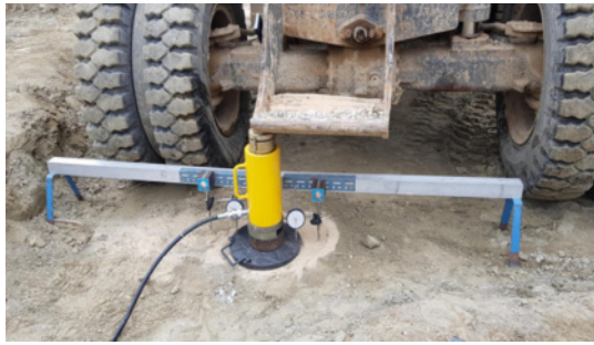
Fig. 3. Plate Bearing Test[19]
