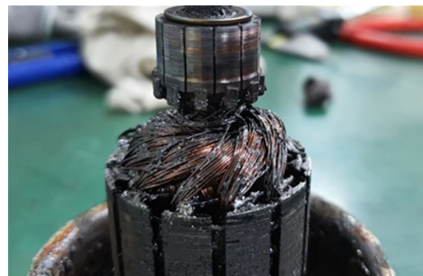
Fig. 12. Damaged rotor by overheating
