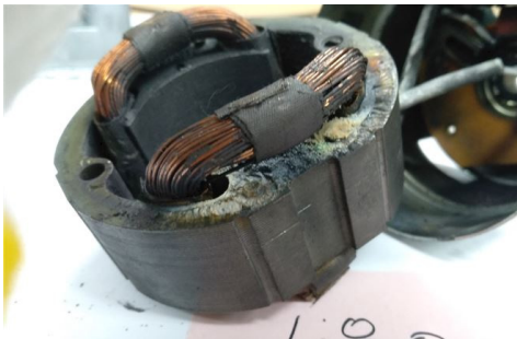
Fig. 3. Damaged stator winding of fuel pump
