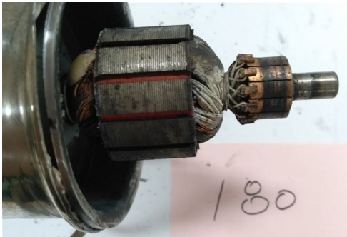
Fig. 4. Damaged rotor winding of fuel pump
