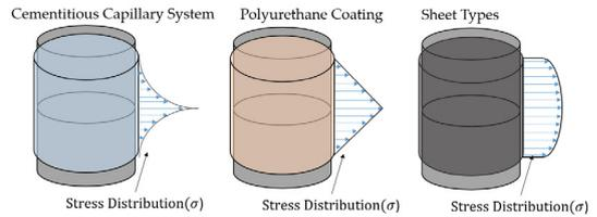
Fig. 7. Stress distribution image of the waterproofing membrane types
