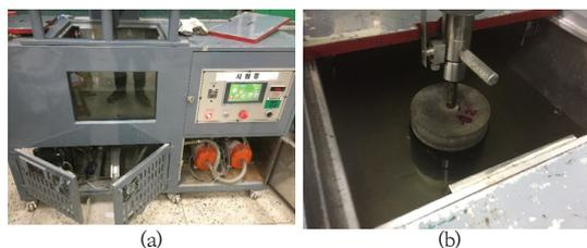
Fig. 4. Testing apparatus illustrated (a) Overview of the joint displacement simulation water chamber; (b) Specimen installed in the joint displacement simulation water chamber
