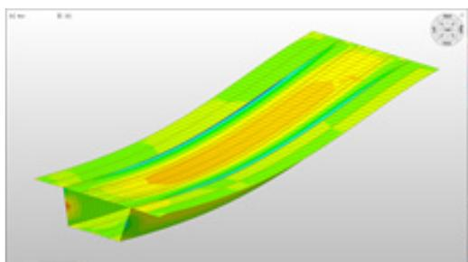
Fig. 2. FEM analysis of the load conditions of waterproofing membrane and concrete railroad bridge deck
