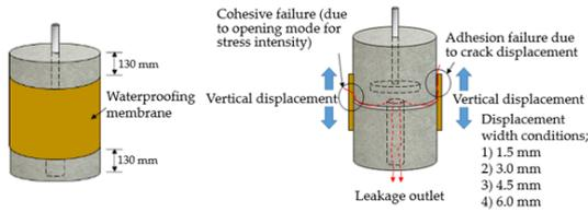
Fig. 3. Crack displacement testing specimen
