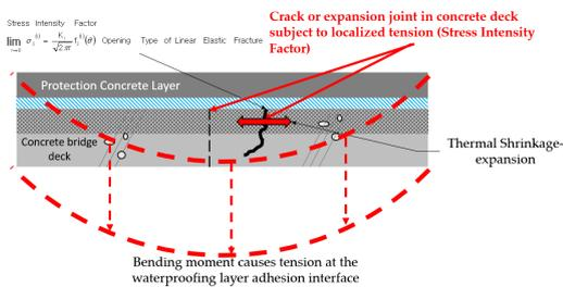
Fig. 6. Stress factors of a bridge deck
