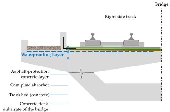
Fig. 1. Sample PSC track bed structure design layout with waterproofing system
