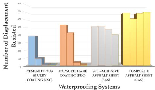
Fig. 5. Joint displacement resistance performance result of the respective waterproofing system types (Per waterproofing system type)
