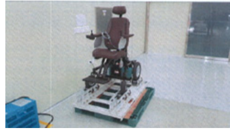
Fig. 9. Jig and electric wheelchair used to measure continuous travel time
