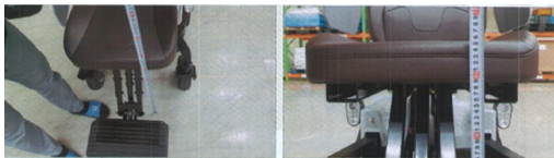
Fig. 12. Maximum lifting height measurement experiment
