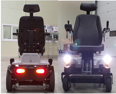
Fig. 7. Application of headlights, turn signals, and car lights when driving at night
