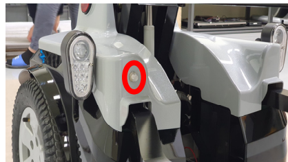
Fig. 6. Application of circuit breaker for power off during over current operation
