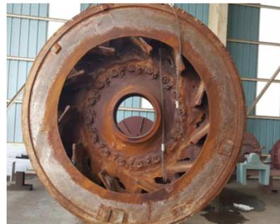
Fig. 2. Erosion of Kiln I.D. blower (S company).
