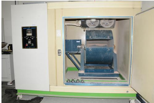
Fig. 2. LA Abrasion Tester in Constant Temperature Chamber
