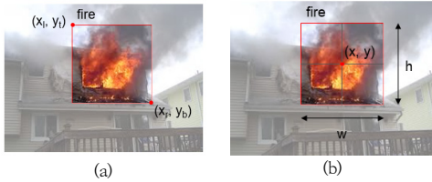
Fig. 2. Image labeling (a) TLBR rectangular coordinate (b) Centroid rectangular coordinate
