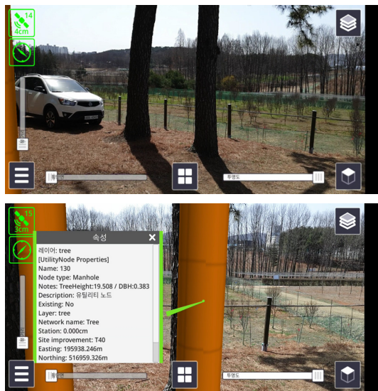
Fig. 11. Tree monitoring using GNSS and AR
