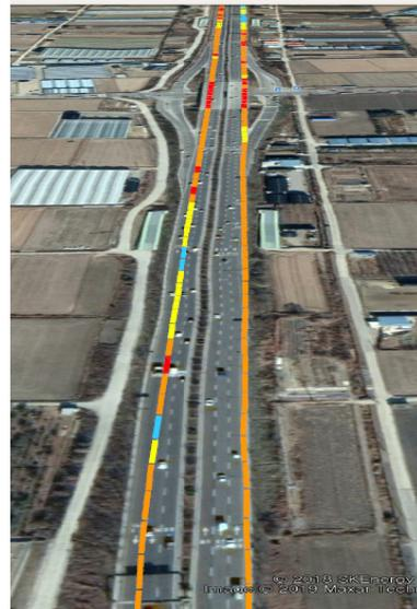
Fig. 5. Visualization of pavement condition rating
