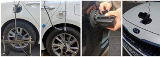
Fig. 4. Proto-type production (Case: On-board type microphone & DMI mount, and multi-channel cam)
