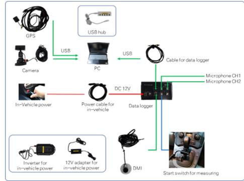
Fig. 2. System architecture of tire-surface noise measurement and processing system
