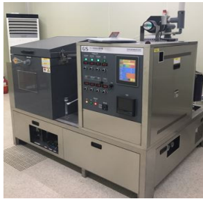
Fig. 4. Gas Corrosion Test Instrument (GS-UVZ)
