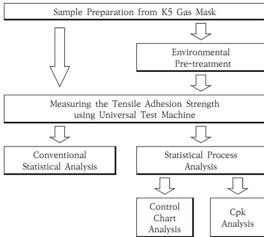
Fig. 2. The schematic diagram of research process.
