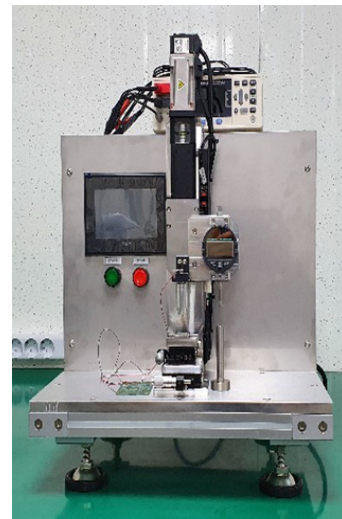
Fig. 8. Test Device for improving test speed and repeat precision
