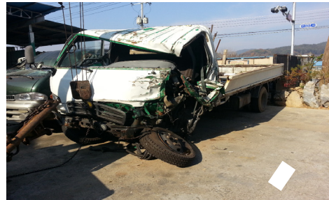
Fig. 7. Mighty left front folded and dislocated front axle and tire deflated left front wheel
