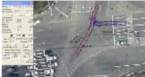
Fig. 7. Sonatas and Lexus have collisions, but they do not match the final stop
