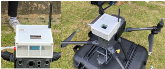
Fig. 1. Measurement module made of 3D printing
