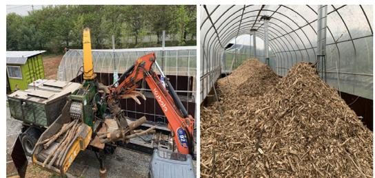
Fig. 4. Netherlands Dutch Dragon EC 6060 Shredder work scene(left), Wood chips loaded by sample(Right)
