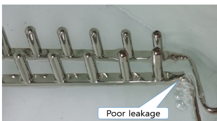
Fig. 4. Poor leakage phenomenon
